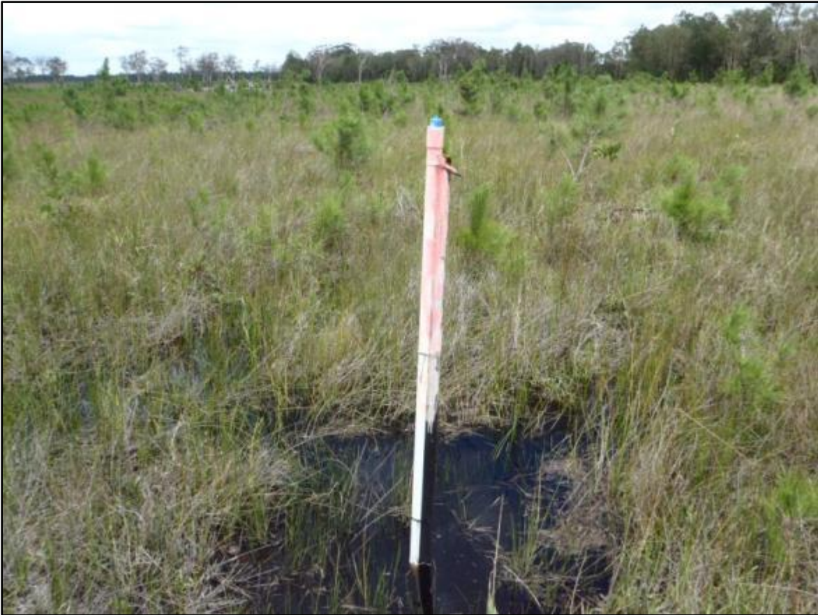
Figure A.2b: Example of water level sensor deployment
