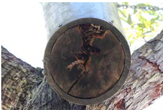
Figure 13: Rotted wooden base of artificial hollow.
