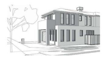
Non-compliant evaporative cooler unit located at side of roof and above roof ridgeline
