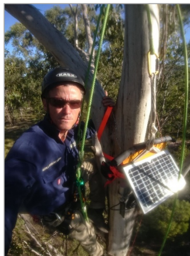
Figure 4. Images showing the installation of a new solar-powered LX base station, high up a gum-topped box. The base station was fastened to the tree using heavy-duty ratchet straps and high tensile wire.
