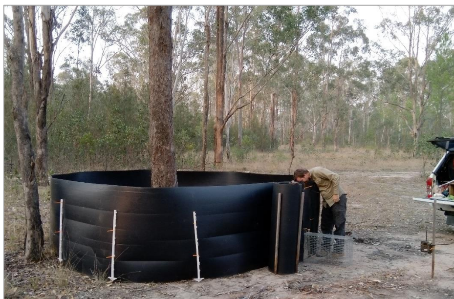
Figure 2. Image of a fence trap set up around an isolated tree to try and catch a koala; an SMS motion-sensor camera (bottom right) was used to send an immediate alert if the koala entered the trap.
