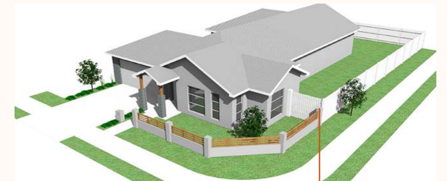
A corner block front fence returning to side fence which stops 4m behind front wall
