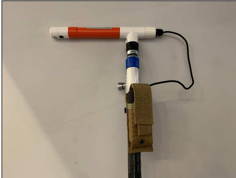
Photo 1: StarWeb Inspection Camera.
