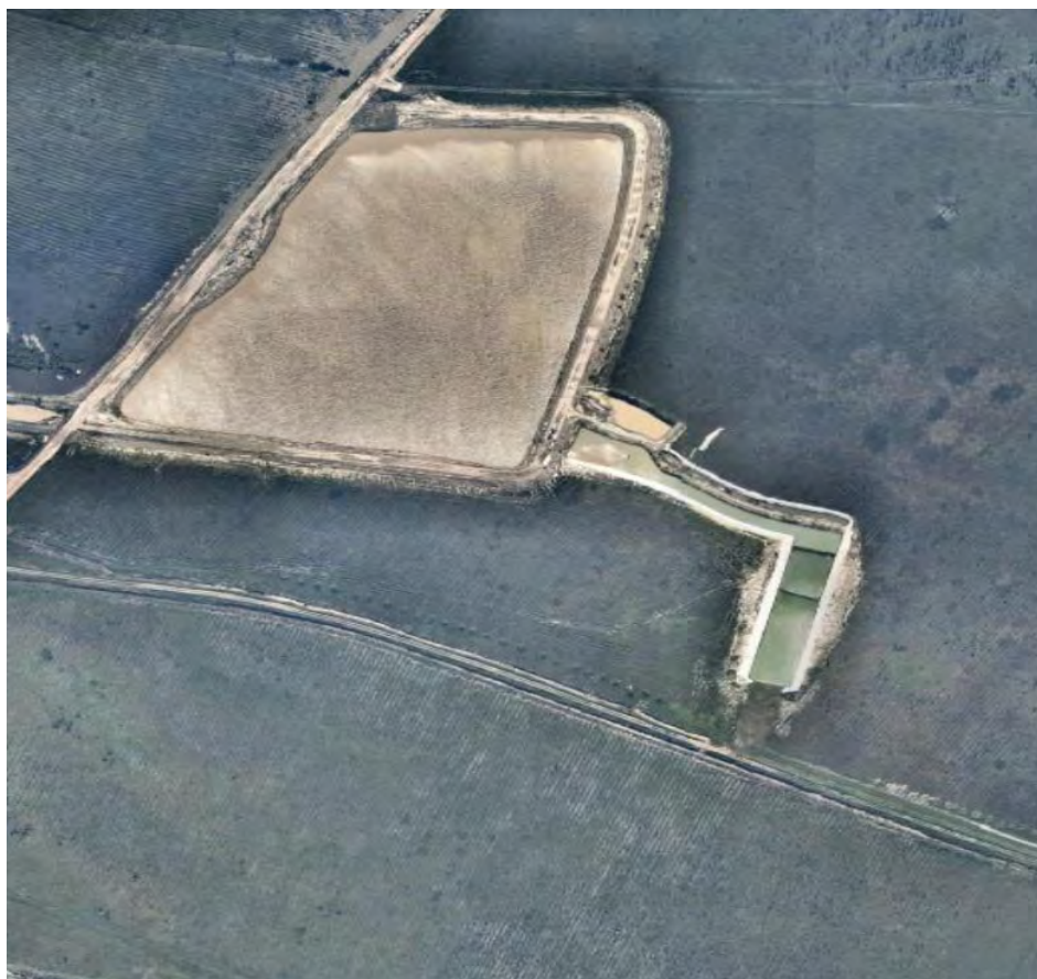
Figure 7: High efficiency sediment basin installed as part of Precinct 7-10 works
