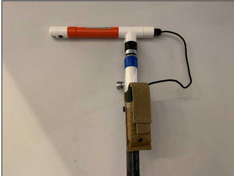
Photo 1: StarWeb Inspection Camera.
