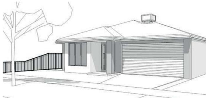
⊗ Non-compliant evaporative cooler unit located at front of roof and above roof ridgeline
